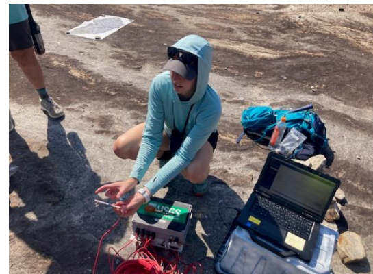
Figure 3-Aislin displays one of the stressmeters from the control borehole.
