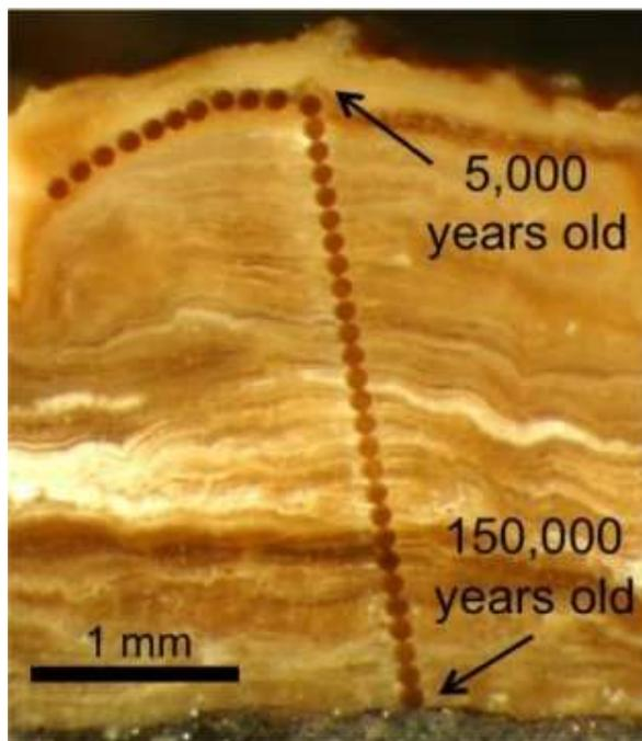
This is a magnified photograph of a cross-section through a 3 mm-thick pedothem soil deposit from Wyoming. The line of dots are laser ablation sampling spots that are 0.1 mm in diameter. The innermost mineral material is about 150,000 years old, and becomes progressively younger towards the outside.
