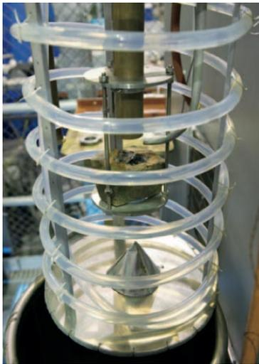
*In this setup, a gyrotron at the top sends a continuous millimeter-wave beam through the copper tube toward the rock sample at the center, and water flows through the surrounding coil. During operation, the device is lowered into the steel chamber below and sealed. Based on the flow volume and temperature rise of the water, the researchers can deduce how much of the incoming energy is absorbed by the rock. Photo: Justin Knight*
