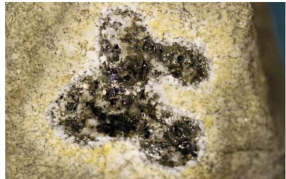
*The dark pattern on this granite sample shows where the beam hit the rock, causing it to bubble and vaporize. The new setup enabled the team not only to vaporize rock for the first time but also to take real-time measurements that provided new insights into key thermodynamic properties of rock up to extremely high temperatures. Photo: Justin Knight*
